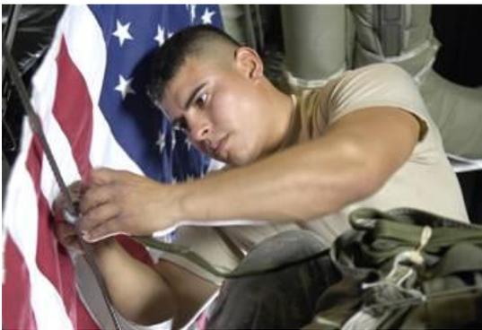
Army Spc. Oscar Osorio attaches the parachute activation cord of a Joint Precision Air Drop System bundle to a C-130 Hercules static line before an airdrop over Afghanistan Aug. 31. Specialist Copley is a parachute rigger with the 647th Quartermaster Detachment. (U.S. Air Force photo/Senior Airman Brian Ferguson)
