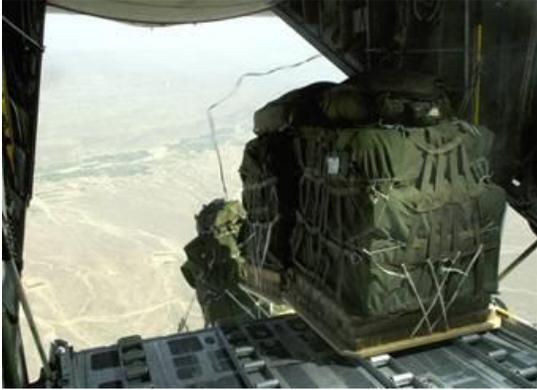
Joint Precision Air Drop System bundles fall out of the back of a C-130 Hercules Aug. 25. The drop was made from almost 10,000 feet above sea level and was calculated using up-to-the-minute wind data relayed from two small dropsondes deployed 20 minutes earlier. The dropsondes calculate wind speed and relay the information back to the aircraft, helping to calculate the correct drop point. (U.S. Air Force photo/Senior Airman Brian Ferguson)
