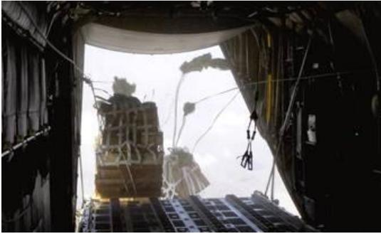
Joint Precision Air Drop System bundles fall out of the back of a C-130 Hercules Aug. 25. The drop was made from almost 10,000 feet above sea level and was calculated using up-to-the-minute wind data relayed from two small dropsondes deployed 20 minutes earlier. The dropsondes calculate wind speed and relay the information back to the aircraft, helping to calculate the correct drop point. (U.S. Air Force photo/Senior Airman Brian Ferguson)
