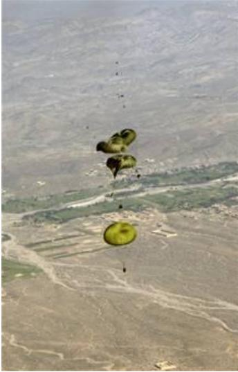
Joint Precision Air Drop System bundles float to the ground after being dropped from a C-130 Hercules Aug. 26. The drop was made from almost 10,000 feet above sea level and was calculated using up-to-the-minute wind data relayed from two small dropsondes deployed 20 minutes earlier. The dropsondes calculate wind speed and relay the information back to the aircraft, helping to calculate the correct drop point. (U.S. Air Force photo/Senior Airman Brian Ferguson)
