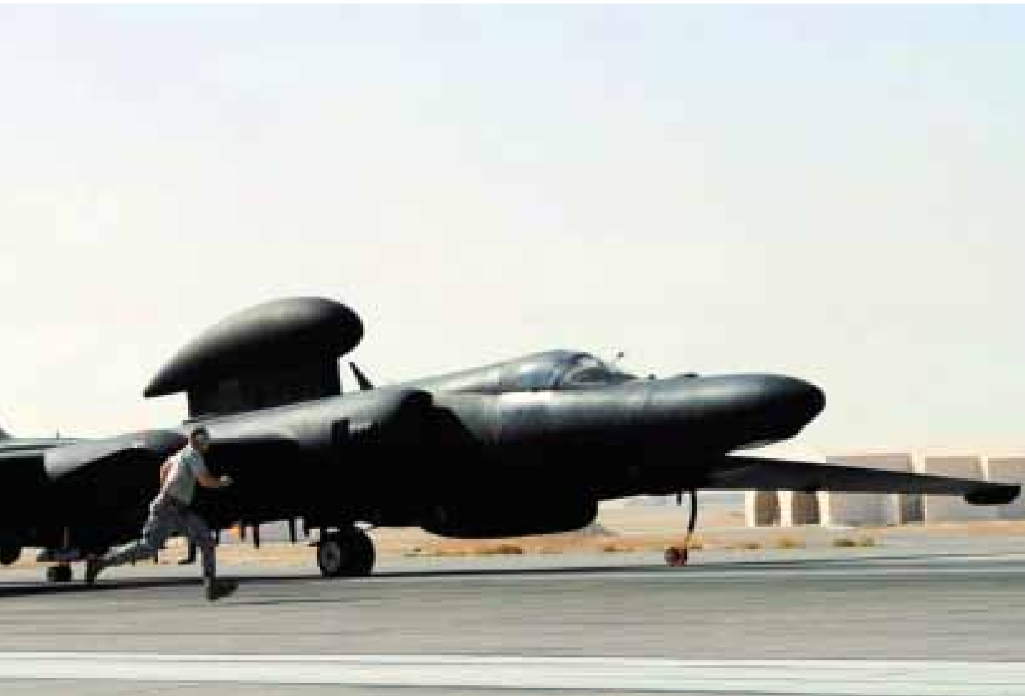
At an unidentified Persian Gulf air base, two USAF airmen prep a U-2S spyplane for imminent takeoff. The aircraft and pilot, Capt. Peter Gryn, were deployed from Beale AFB, Calif., to the 380th Air Expeditionary Wing. U-2s, with a wingspan of 103 feet, can fly above 70,000 feet to provide intelligence-surveillance-reconnaissance data for combatant commanders and individual troops alike. This particular U-2, No. 68-10337, exceeded 25,000 flying hours on a mission flown two weeks after this photo was snapped.
