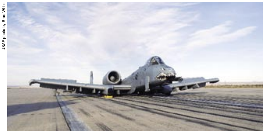
Wheels Up: An A-10 from the 75th Fighter Squadron, Moody AFB, Ga., rests on the runway at Edwards AFB, Calif., after a March 25 emergency landing. The Warthog crash-landed with its landing gear in the up position after the pilot declared an in-flight emergency during a Green Flag sortie. The pilot was uninjured.
