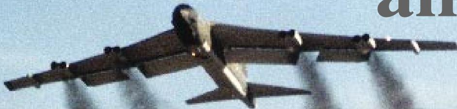
*Strategic Air Command B-52s launch seconds apart, demonstrating the MITO—minimum interval takeoff—formation capability needed to respond to a combat alert.*
