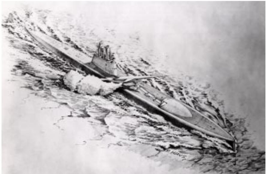
**The Navy for some years investigated ideas for aircraft-carrying submarines. Pictured is a 1957 Navy concept for a 346-foot, nuclear-powered submarine capable of launching large Regulus II cruise missiles from the deck.**
