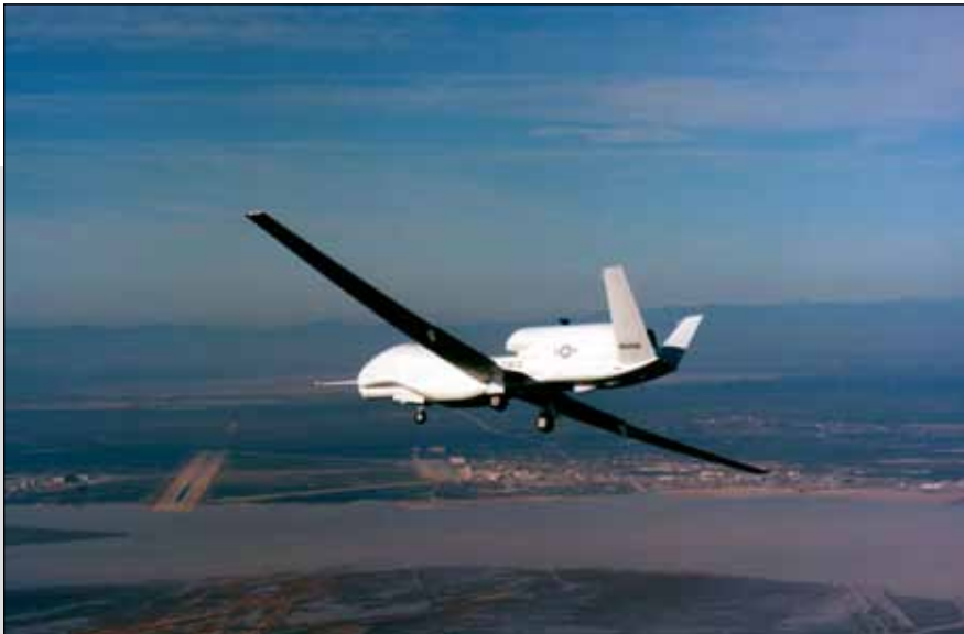
The Air Force is moving toward pervasive Intelligence, Surveillance, and Reconnaissance, meaning uninterrupted watching of areas of interest. The Global Hawk drone can stay high over a hot spot for 24 hours, its sensors glued to the target.
