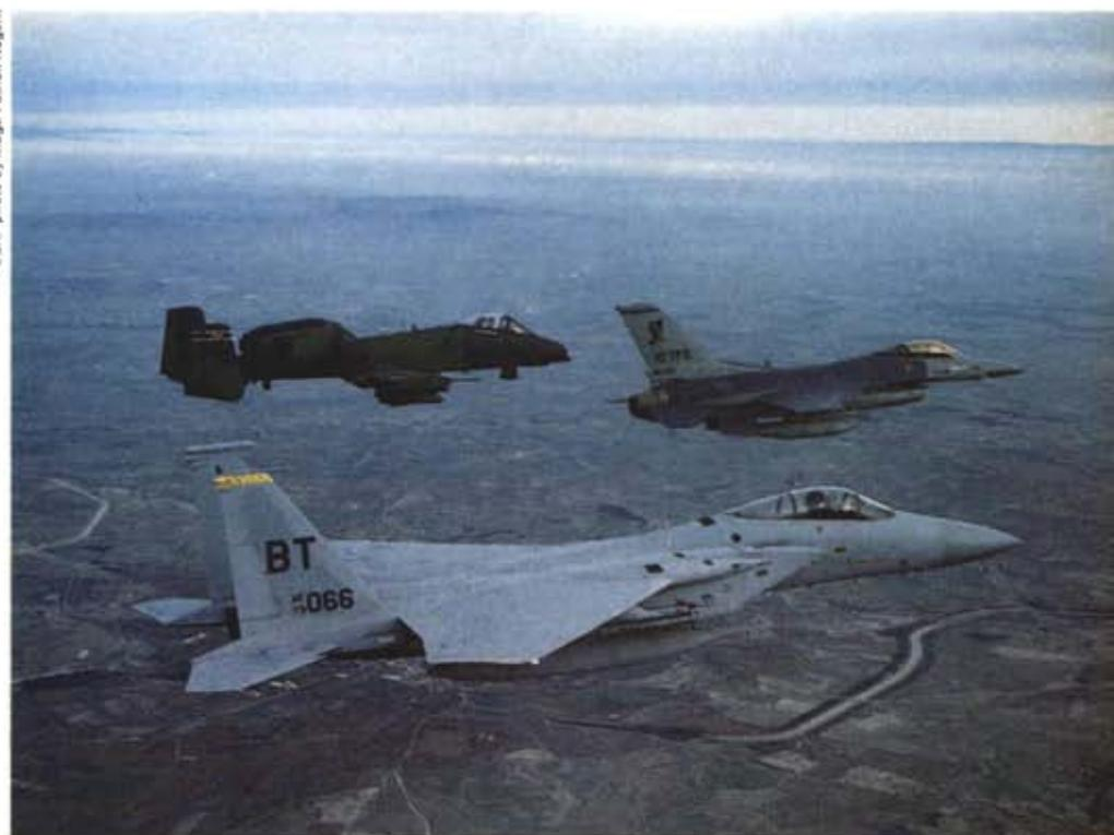
*For purposes of argument, the Air Force's mission breaks down into air superiority, represented by the F-15 (foreground), air interdiction, as shown by the F-16 (right), and close air support in the form of the A-10. In reality, though, the roles are not so clearly drawn. Over a fluid battlefield, one day's air interdiction could become tomorrow's air support.*
