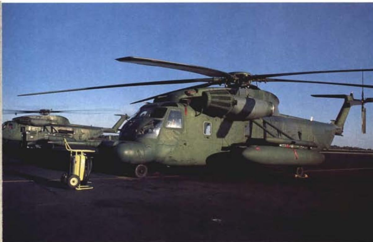
The 1st SOW's specialized rotary-wing assets are the Sikorsky MH-53H Pave Low II helicopters. The Pave Low IIs tend to operate closer to the ground more often than their fixed-wing brethren, so the helicopters are beefed up with 1,000 pounds of armor plate and are able to hover automatically. The helicopter in the background is a transient CH-53B.
